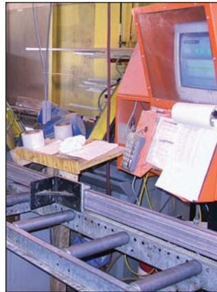
model that can be networked or the cut list can be copied to a disk that is inserted at the saw. This model is a little more costly than some others. Mango has recently come out with the same measuring stop but the sawyer manually enters the length of the piece from the cut list. This model is fairly inexpensive and eliminates the need to measure and mark each piece.
