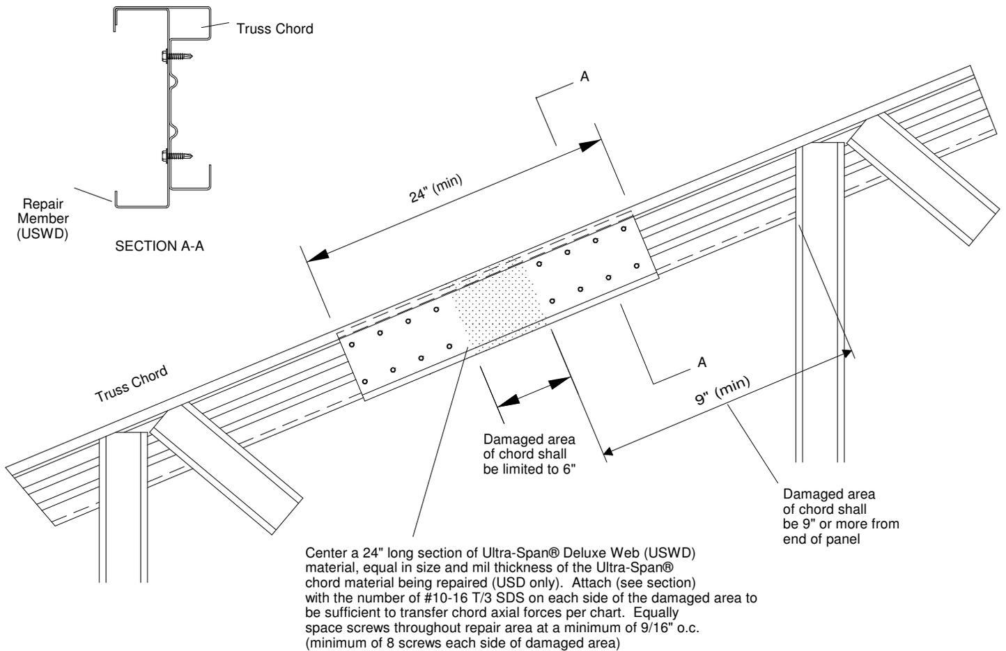
Center a 24" long section of Ultra-Span® Deluxe Web (USWD) material, equal in size and mil thickness of the Ultra-Span® chord material being repaired (USD only). Attach (see section) with the number of #10-16 T/3 SDS on each side of the damaged area to be sufficient to transfer chord axial forces per chart. Equally space screws throughout repair area at a minimum of 9/16" o.c. (minimum of 8 screws each side of damaged area)
